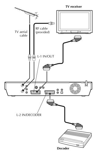
The L-2 IN/DECODER connector can be used as an input connector for an external decoder (descrambler). Simply connect a decoder and you can enjoy a variety of programming that is available through scrambled channels.
